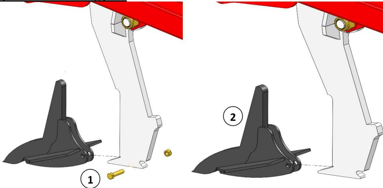
**Before working with the wearing points, the machine must be secured. This can be performed by placing trestles under the main frame or by supporting the roller.**
