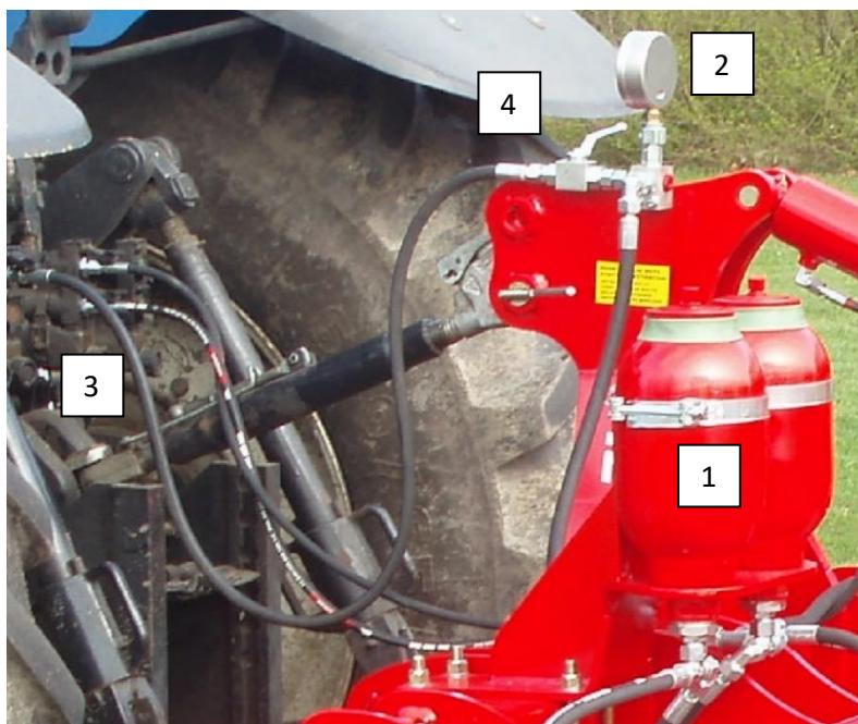
1. Before each season it has to be controlled, that the gas pressure in the accumulator (Pos.1) is 110 bars. **!** This requires special tools and can only be performed by an authorized dealer.
