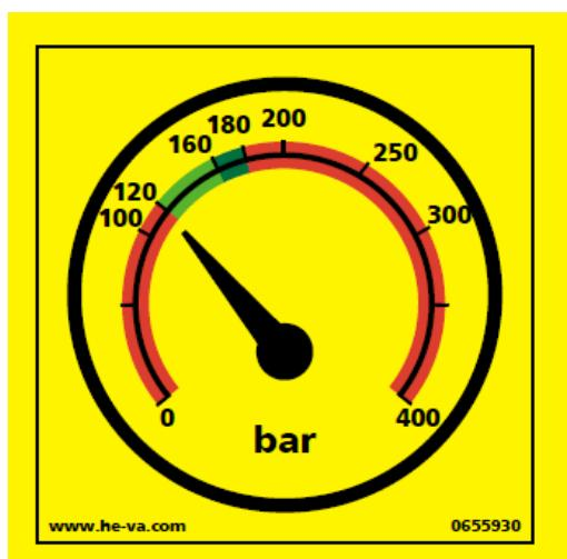
Correct hydraulic pressure on the release system
